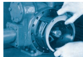
Easily replaceable liner restores efficiency.
